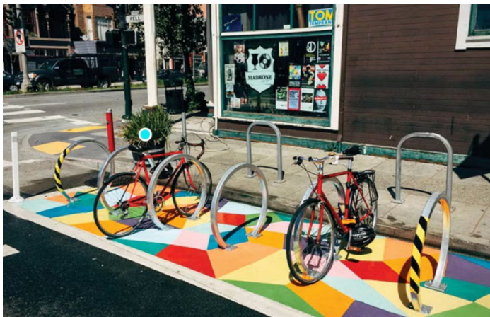
Figure 1: Example of a curb with painted daylighting and bike racks
