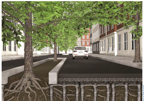
Trees stunted by surrounding compacted soil (top) can grow as intended by using structured soil or Silva cells (below).
